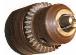
Keyed chuck showing the three clamping jaws.
