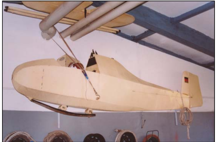
The Hutter fuse, elevator and struts.
