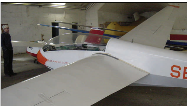
An example of a Swedish Bergfalke with a new, highly modified, one piece canopy design. The headroom is improved by raising the height of the canopy over the pilot's heads, as well as being significantly wider near the top of the canopy. The visibility is improved by removing the join between the front and rear pieces. Whilst the above example improves both visibility and headroom, it also requires significant modification of the fuselage and the nose in order to fit it. The club hopes to incorporate some of these improvements whilst not modifying the fuselage or the nose of GZM.
