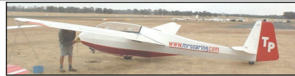
A Bergfalke III, VH-GTP, owned by Ian McPhee of Byron Bay, NSW. It was fitted with a one piece canopy that was manufactured in England in the mid 1980s. This one-piece design improves the visibility, particularly for the rear pilot. However the canopy has the original cross section and does not improve the headroom.
