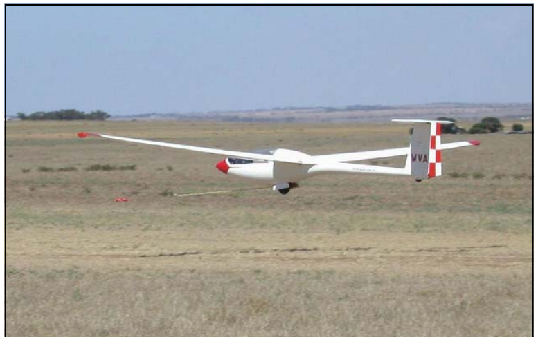
The club's Pik 20D in initial climb on a winching cable. As the glider gains more height and speed the pilot will rotate to a standard climb angle of 45°.
