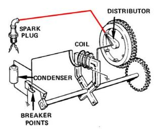
Just the same as cars, the magneto points also have a capacitor (some people still call them condensers) across the points. The capacitor is used to both extend breaker contact life by diverting current away from the points during switching and it also increases the induced voltage to give a more powerful spark.
