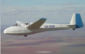
**The Puchatek (KRO):** This is a Polish-built, aluminium two-seater that was bought brand new by the club back in 1994. Whilst only of average performance, it is excellent for basic flight training and also has the advantage of being rated for aerobatics for those that tire of straight-and-level flight. Puchatek (pronounced "Pooka-tek") apparently is Polish for 'fluffy bear' and is their nick-name for 'Winnie the Pooh'.
