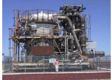
We also went to EBR1. It was the world's first nuclear power station. During the cold war the Russians convinced the US that they had a nuclear powered jet. So the Americans built a nuclear jet engine. It was not small, and weighed several tons. Boeing had plans to build the plane, including several tons of lead shielding to protect the pilots. They had the hangar built and were planning a 20 mile runway when Kennedy scrapped it. Only in America.
