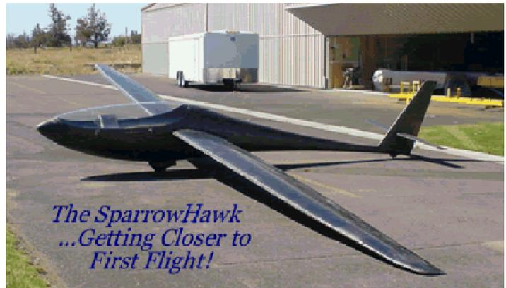
Windward Performance is designing and building a high performance ultralight (FAR Part 103 legal) sailplane called the *SparrowHawk*. It is completely manufactured from oven cured carbon epoxy prepreg and will be finished in polyurethane. The manufacturers promise it to be a quick and nimble aircraft with a very low sink rate.
