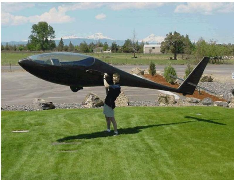
The Sparrow Hawk should be readily easy to rig as the wings only weigh 20 kg each. The fuselage weighs in at an impressive 34 kg as demonstrated in the photo on the left.
