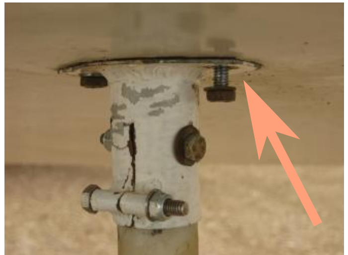
When DI'ing the MotorFalke always check that the bolts holding the wing walker legs in are tight and secure!
