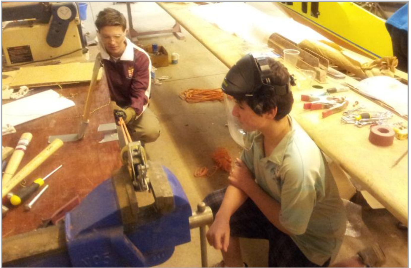
Michael and Peter Conway undertake release testing of a K-13 back release - one down, four more to go... (on a serious note, its good to see that both are using protective equipment when performing the test as the process required the release to be placed under considerable load.)
