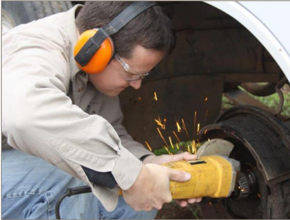
Leigh applies some tough love to the recalcitrant wheel bearing which had welded itself to the shaft.
