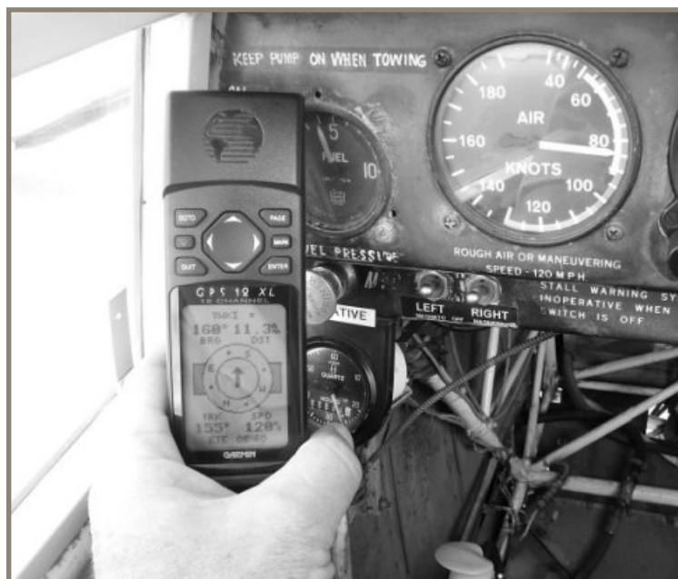
The tug ferry home had a ferocious tail wind - the ASI reads 85 kts and the GPS shows a ground speed of 120 kts. (Photo P. Siddall).
