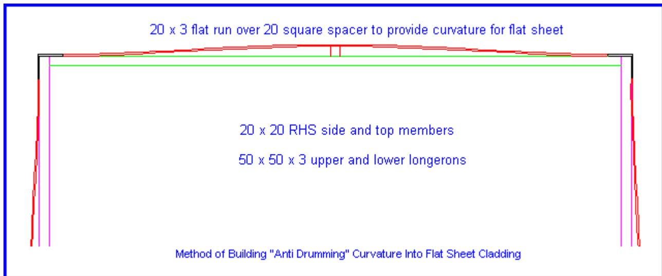
When galvanised steel sheet is used it can be procured with either a natural galvanised finish or with a colorbonded finish. White colorbond is worth the additional cost since it eliminates the need to paint the trailer.
