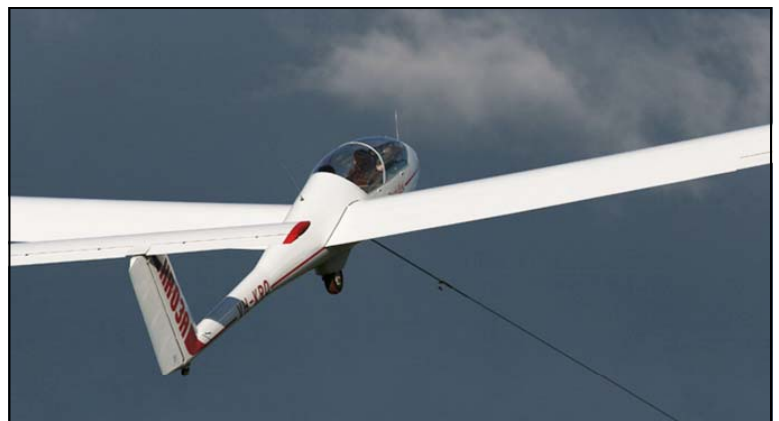
That's me flying the Puchatek from the front seat. I'm looking at the port wing to see if I've established full climb, which should mean that the glider is at a 45° angle to the ground. Photo: Jeff Philcox
