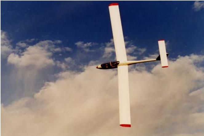
**The Puchatek (KRO):** This is a Polish-built, aluminium two-seater that was bought brand new by the club back in 1994. Whilst only of average performance, it is excellent for basic flight training and also has the advantage of being rated for aerobatics for those that tire of straight-and-level flight. Puchatek (pronounced "Pooka-tek") apparently is Polish for 'fluffy bear' and is their nick-name for 'Winnie the Pooh'.
